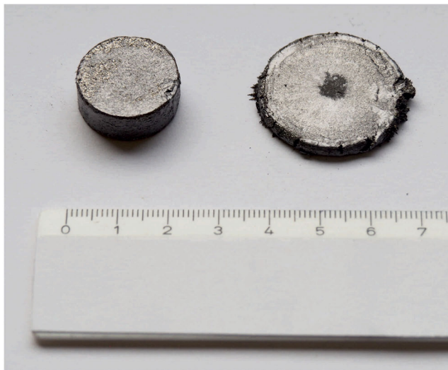
Figure 3. NdFeB samples after presintering by FAST/SPS ( 100 \text{ K min}^{-1} , 50 MPa, 500 °C, 30 s) and after deformation by flash SPS (MQU-F1_5, 32 MPa, 35 kW, 30 s).
